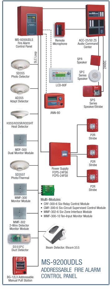
**MMF-300:** Addressable Monitor Module for one zone of normally-open dry-contact initiating devices. Mounts in standard 4.0" (10.16 cm.) box. Includes plastic cover plate and end-of-line resistor. Module may be configured for either a Style B (Class B) or Style D (Class A) IDC.
